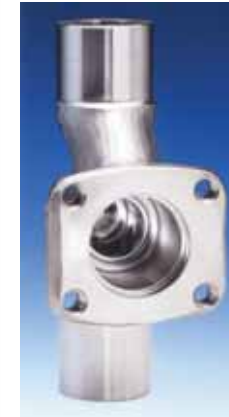
Stainless steel valve body, internally electropolished to produce a clean, particle free surface
