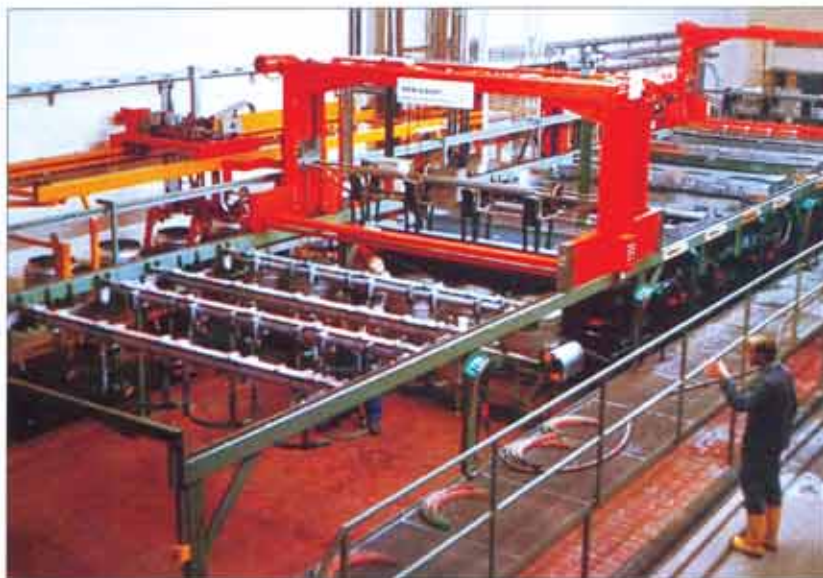
Full automated Poligrat plant type EK3500AS for electropolishing stainless steel drums for spin dryers
